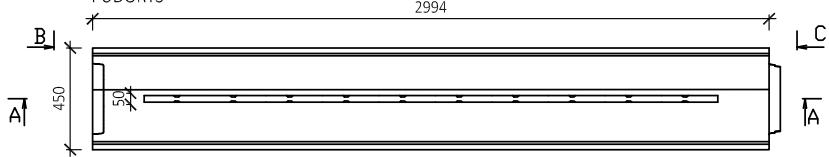
BEST TROUBA S PRŮBĚŽNÝM ŠTĚRBINOVÝM ŽLABEM 2 m, OBRUBNÍK 7 cm (PROFIL PRAVÝ)
