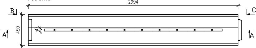
BEST TROUBA S PRŮBĚŽNÝM ŠTĚRBINOVÝM ŽLABEM 2 m, OBRUBNÍK 15 cm (PROFIL PRAVÝ)
