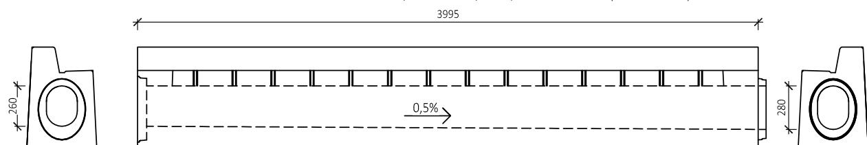
BEST TROUBA S PRŮBĚŽNÝM ŠTĚRBINOVÝM ŽLABEM, SPÁDOVÁ 20/24-26, OBRUBNÍK 15 cm (PROFIL PRAVÝ)
