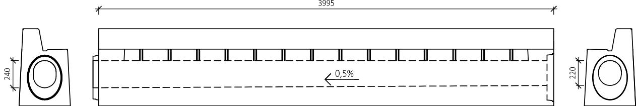
BEST TROUBA S PRŮBĚŽNÝM ŠTĚRBINOVÝM ŽLABEM, SPÁDOVÁ 20/20-22, OBRUBNÍK 18 cm (PROFIL LEVÝ)
